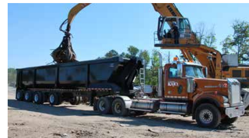
Frameless full width draft arms. All wheels stay on ground
