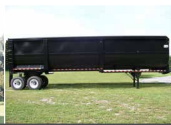
Frameless full width draft arms. All wheels stay on ground
